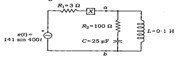
(i) Find the equivalent impedance appearing to the right of points ab.
