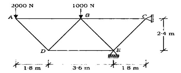
(b) Three members of the truss shown in the figure below have been cut either too long (+ve) or too short (-ve) as per details given below. Calculate the vertical displacement of joint D due to discrepancies in the length of these members by unit load method.
