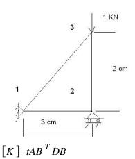
$$D = \frac{E}{1-\mu^{2}} \begin{bmatrix} 1 & \mu & 0 \\ \mu & 1 & 0 \\ 0 & 0 & \frac{1-\mu}{2} \end{bmatrix}$$
