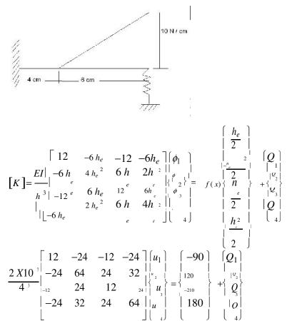
$U_1 = 0.0001 \text{ mm}, U_2 = 0.0001 \text{ mm}, U_3 = 0.0001 \text{ mm}, U_4 = 0.0001 \text{ mm}$
