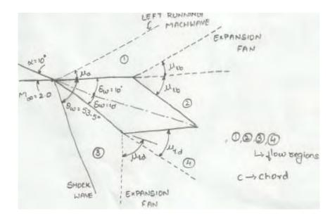
8. The geometry of a double wedge airfoil section is as shown in figure
