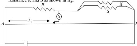
When an unknown resistance X is connected in parallel with the resistance S, the balance point slifts to a distance  $\ell_2$ . Find the expression for X in terms of  $\ell_1$   $\ell_2$  and S.
