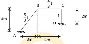
If the final moment at B is 100 kN m, then the moment developed at end A is (A) 23KN-m (B) 24KN-m (C) 25KN-m (D) 26KN-m
