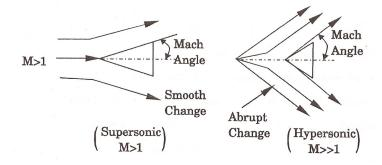
Mach angle is formed, when an object is moving with supersonic speed. The wave propagation and changes are smooth. When an object is moving with hypersonic speed the changes are abrupt is shown in Fig. Hence for a supersonic flow over two – dimensional object "mach wedge" is used instead of "mach cone".
