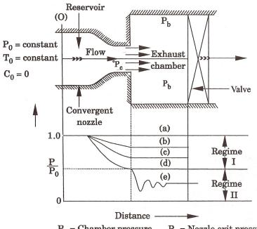
$P_{\rm b}$  = Chamber pressure  $P_{\rm e}$  = Nozzle exit pressu Isentropic flow through a convergent nozzle
