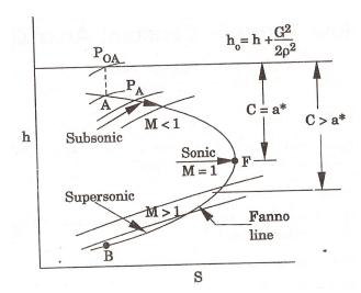
The equation which yields the fanno line for the given values of  $h_0$  and G is called "fanno flow equation".
