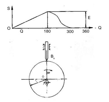
b) Name the following mechanism and explain it's working principle. 6
