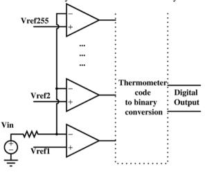
If the flash ADC has 8 bit resolution, which one of the following alternatives is closest to the maximum sampling rate ?
