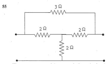
The y<sub>21</sub> parameter of the network shown in the given figure will be
