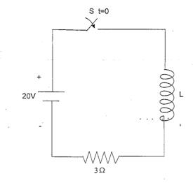
For the circuit shown in the figure, the switch is closed at t=0. After some time when the current in the inductor was 6A, the rate of change of current through the inductor was 4A/sec. The value of the inductor is
