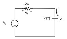
The voltage function is shown below The current i(t) for  $0 < t \le 1$  is
