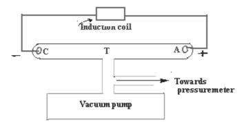
Potential difference of few kilovolts (obtained from an induction coil) is applied between the terminals A and C at normal pressures. The gas is found non conducting at this pressure.
