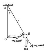
The angular displacement of the sphere due to this torque being of decreasing value it (the torque) is taken as negative.
