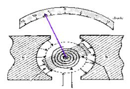
In a galvanometer, between two cylindrical poles of a permanent magnet a light rectangular frame possessing winding of thin copper wire is suspended on frictionless pivot.
