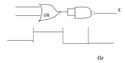
Two car garages have a common gate which needs to open automatically when a car enters either of the garages or car enters both. Design a truth table, logic symbol and hence Boolean expression for a circuit that resembles this situation using diodes.
