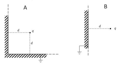
In situation A, two semi-infinite earthed conducting planes meet at right-angles. A point charge q, is placed at a distance d from each plane, as shown in the figure A. The magnitude of the force exerted on the charge q is denoted  $F_A$ .
