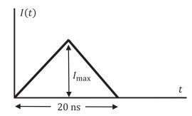
The typical output current, as a function of time, is shown by the figure below for a few pulses, where  $I_{\text{max}}$  is 80  $\mu$ A. It follows that the number of photons in each pulse is
