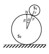
At what minimum value of  $\theta$  will the spheres lose contact?
