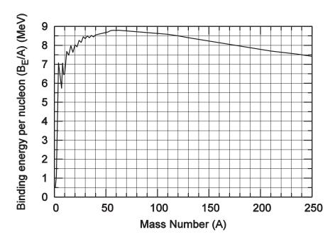
If a nucleus of mass number A=240 undergoes a symmetric fission to two daughter nuclei each of mass number A=120, write down the amount of energy released in this process, in units of MeV, using this theoretical model.
