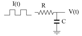
Which of the following represents the correct voltage across the capacitor C?
