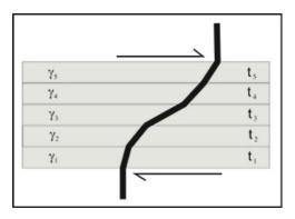
Total shear displacement along the shear zone is given by
