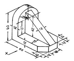
(b) Sketch the two views (top view and front view) of the object shown in the figure. Put the dimensions.
