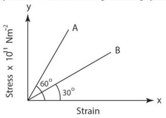
The cross-sectional area of wire A is  $5 mm^2$  whereas that of wire B is  $10 mm^2$ .
