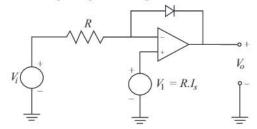
The current through the diode at temperature T is given by:  $I = I_s(e^{\frac{V}{V_T}}-1)$  where V is the forward voltage across the diode and  $V_T$  is the volt equivalent of temperature.
