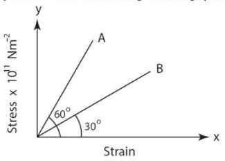
The cross-sectional area of the wire made of A is  $5 \ mm^2$  whereas that of the wire made of B is  $10 \ mm^2$ .
