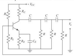
(a) Prove that the frequency of oscillation is given by
